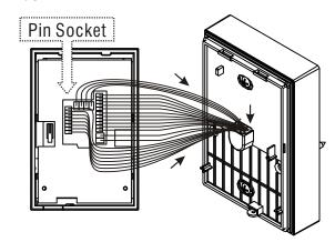
5. Thread the wires thru the cut-out opening on conjunction box.
